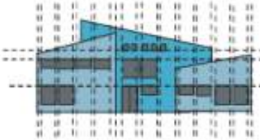
(35) The Regulating Lines of a Building are Invisible Lines that Control the Location of Major Features
