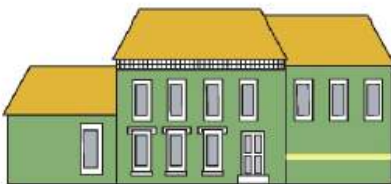
(36) Consistent use of Details on all Sides of a Mass, E. G. Windows Surrounds on all First Floor Windows of the Main Body
